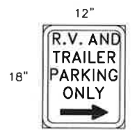
R.V. AND TRAILER (RIGHT) SIGN DETAIL
